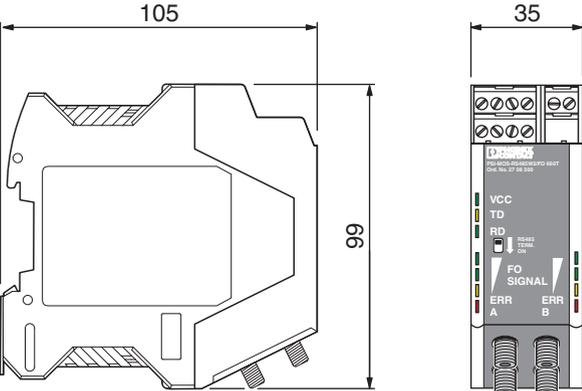
Figure 2 Housing dimensions
