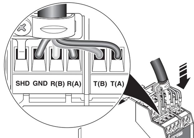
Figure 11 Shield connection
