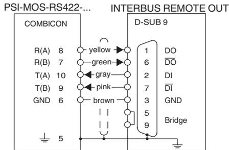
Figure 12 Connection to INTERBUS REMOTE OUT
