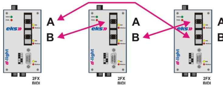
Systems with BIDI transceivers always have to be connected from transceiver type A to a transceiver type B. Switches with 2 FX-Ports always have transceiver type A as the upper one.
