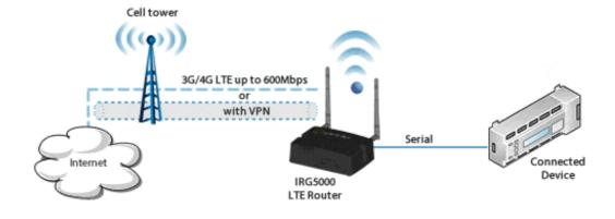
The Perle IRG5000 supports Point-to-Point (PPP) to establish a connection to a host PC serial port. The IRG5000 supports Windows Dial-up Networking when PPP is enabled to establish a connection to a host PC serial port.
