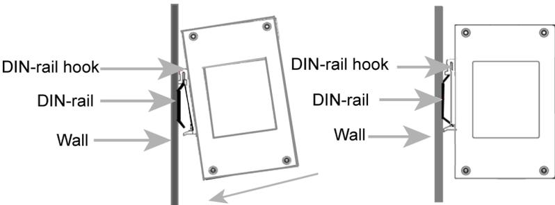
**Note:** To remove the IDS-105G switch from the DIN-rail, push down slightly on the IDS-105G while pulling the bottom out.
